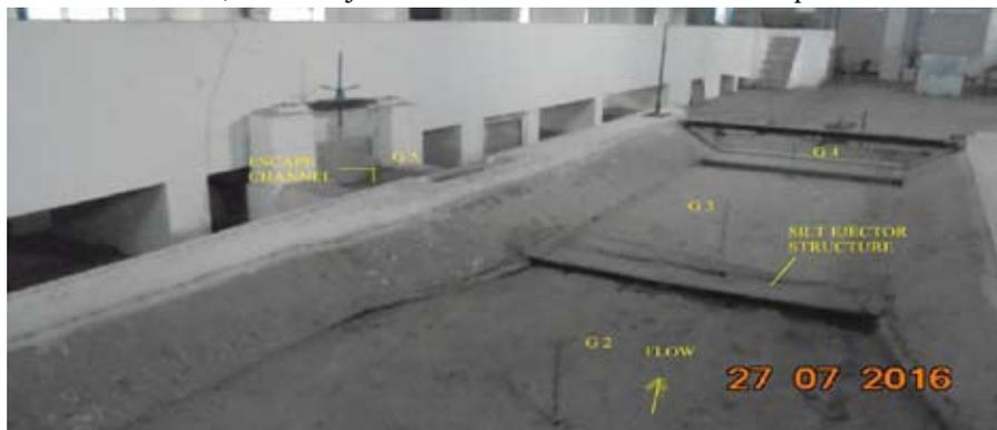
Fig 1 : Photograph of Silt Ejector Model
