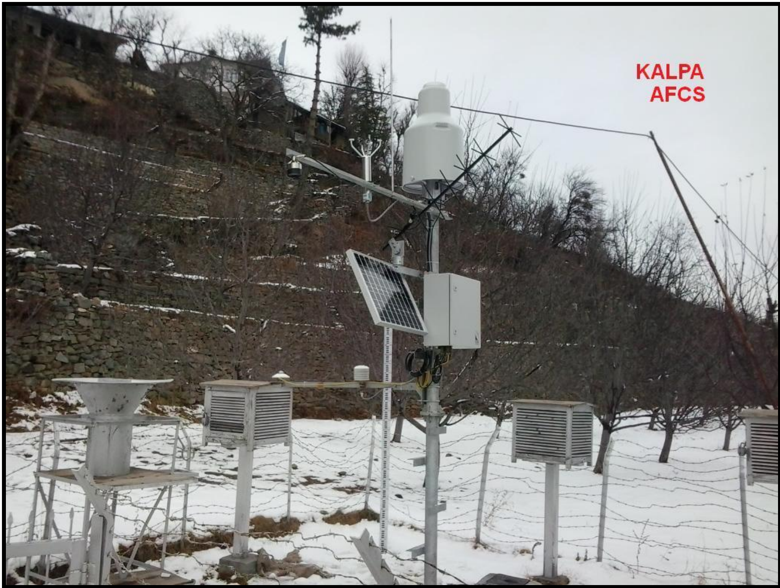
22 Full Climatic Station Installed at Kalpa, Elevation 9046 ft
