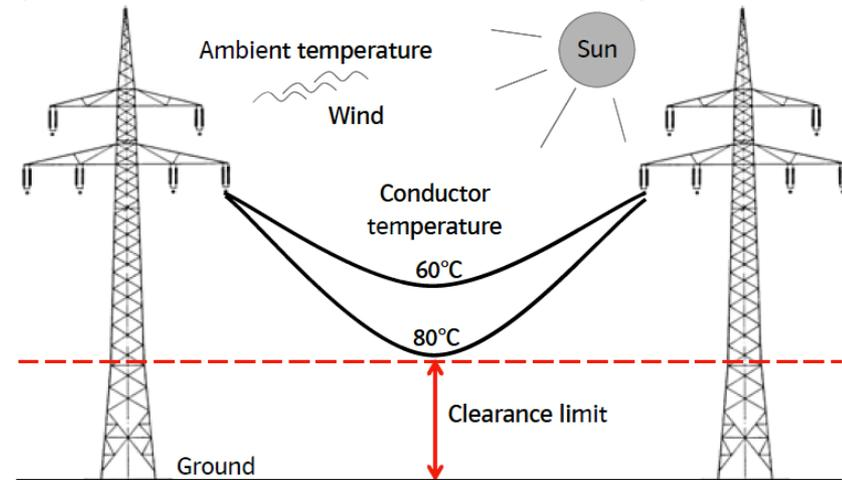
*Figure 1: Clearance depending on ambient conditions and current*
