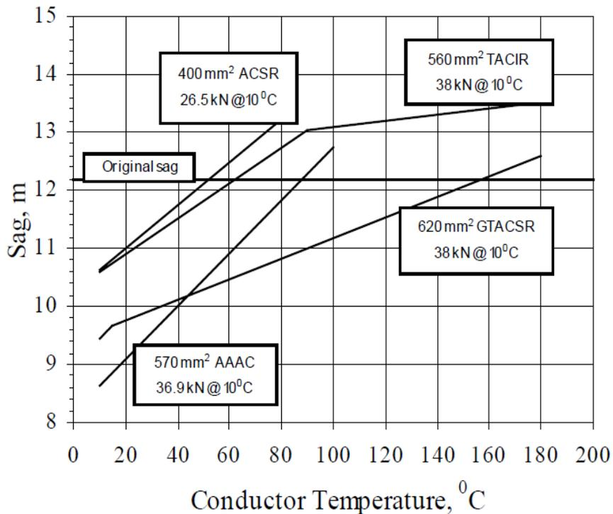
**Next step:** conductors with „knee point“ to reduce the increase of sag with temperature
