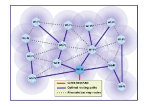
The adjacent figure shall illustrate how the current routing may look like. The network basically needs only a single Gateway connection (red line) towards the backbone/backhaul. For redundancy reasons, a second could be considered and will allow further, fully automatic optimization of the Wi-Fi Mesh.
