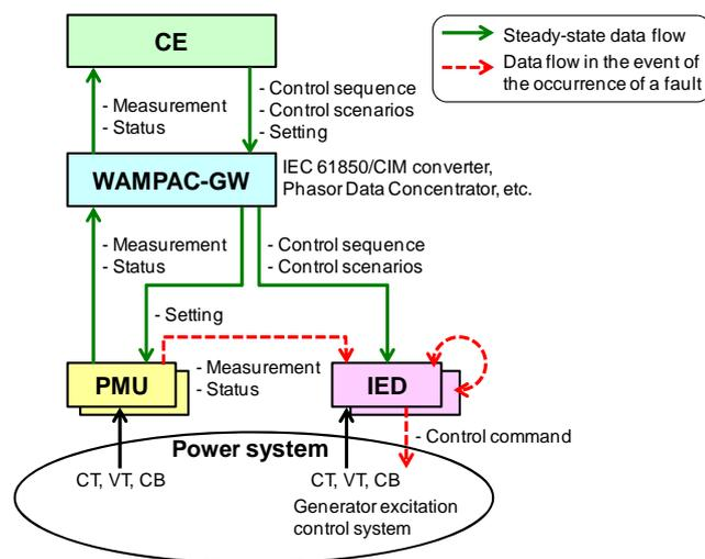
Fig. 1 Proposed WAMPAC system configuration illustrating the operational data flow
