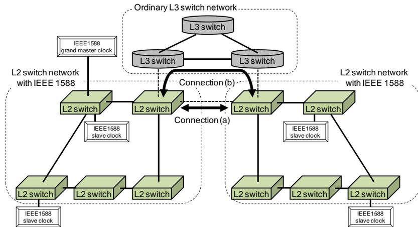
Fig. 4 Experimental configuration of PTP internetworking
