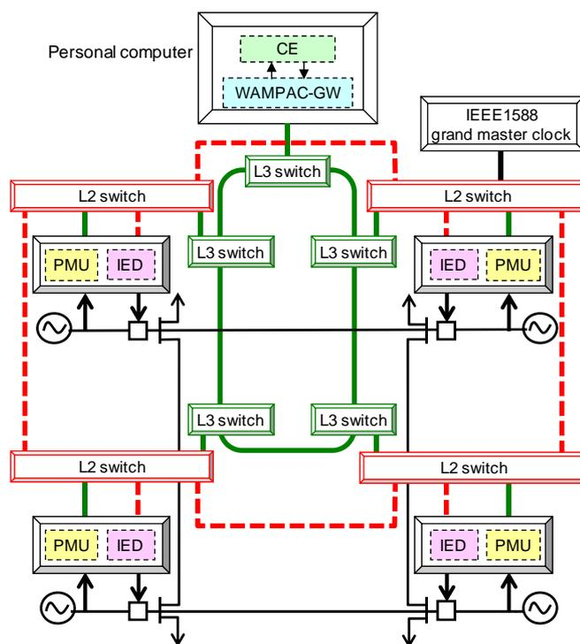
Fig. 6 Configuration of the prototype WAMPAC system
