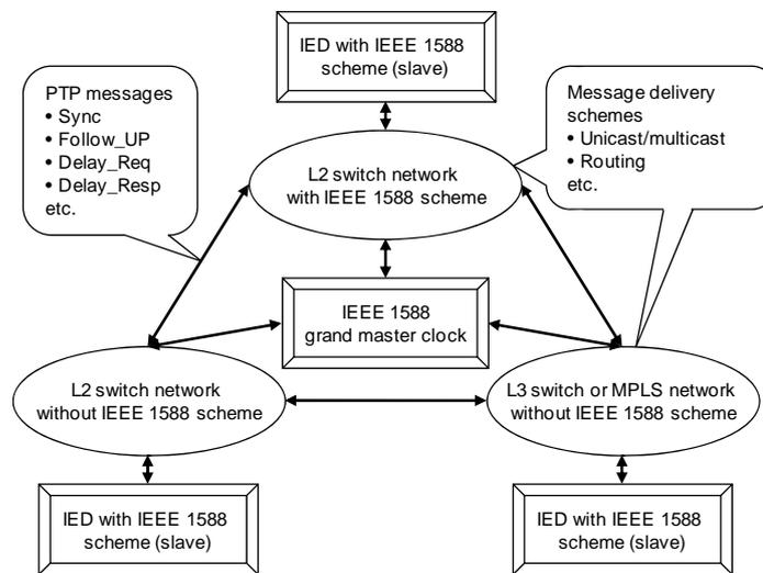
Fig. 3 Internetworking for PTP time synchronization
