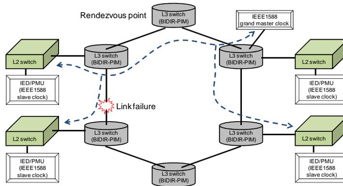
Fig. 5 Experimental configuration of bidirectional IP multicast operation
