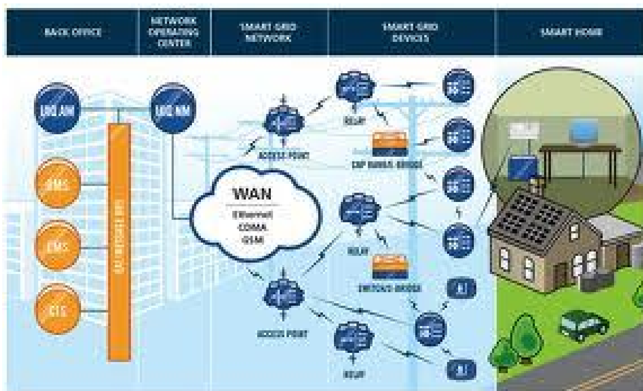
Figure 5 - Smart Grid - Connecting Utilities with the consumer
