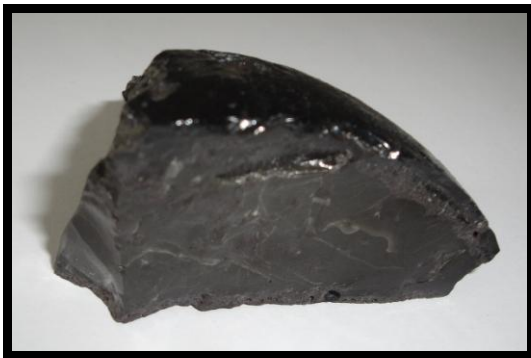
Figures 6 and 7: Al-Li aggregate used in cement and ceramics industry and Cu-Co-Fe-Ni alloy for refining and reuse in the lithium-ion batteries industry (Photos: Alexandre Pinhel - Material provided by SAFT / Umicore - Real Size)
