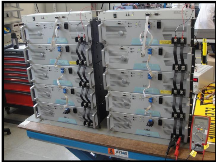
Figures 4 and 5: Tests on lithium-ion batteries in the factory and final installation in the company (Photos: Alexandre Pinhel)
