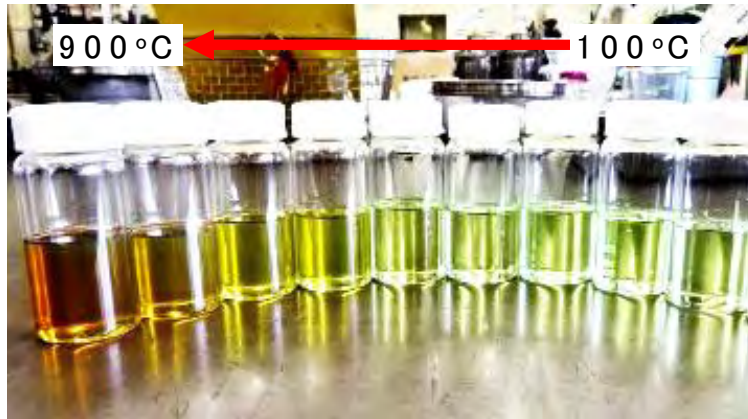
Fig.3 Natural ester oil after heating test
