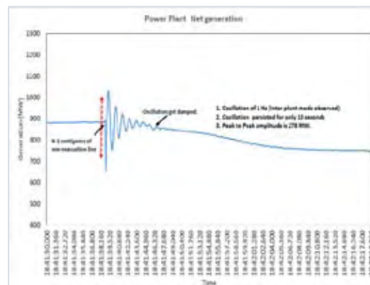
Figure 6: LFO and its damping observed in Power Plant Output at the Power Plant with Properly tuned PSS.
