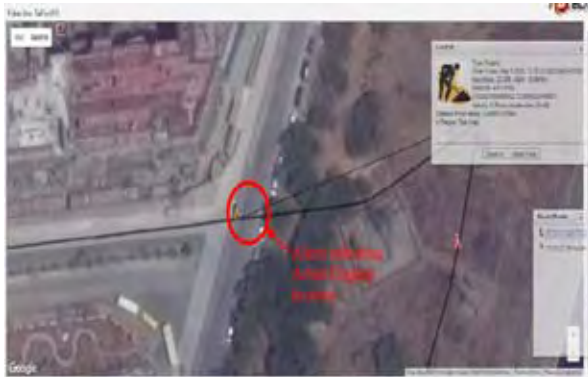
Fig 7- Digging activity detected in real time is available on computers at remote location
