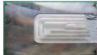
(3) Metallic putty Rusting : None Penetration : None
