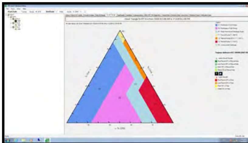
Figure 13 Duval Triangle of Nine-gas DGA On-Line Monitoring System
