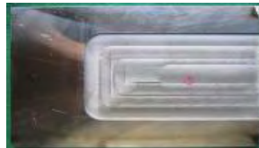
(2) Epoxi putty Rusting : None Penetration : None
