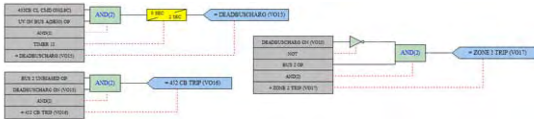
Fig. 7. Logic for tripping only BC & Zone1 for faults in blind spot
