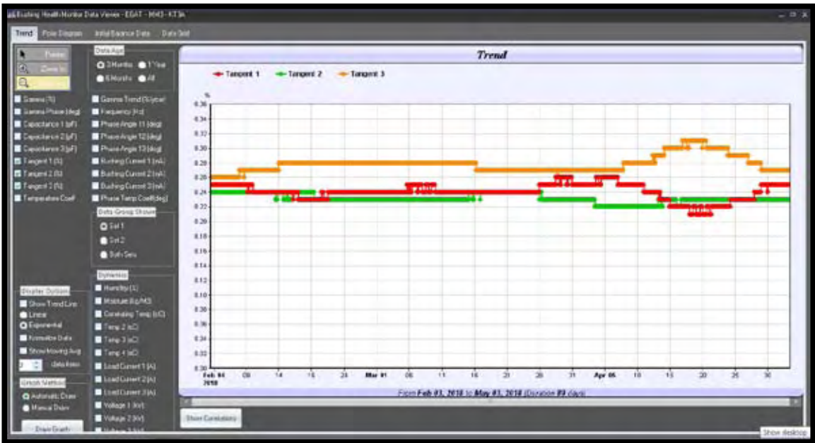
Figure 8 continuous Trend-Tangent delta of Bushing On-Line Monitoring System
