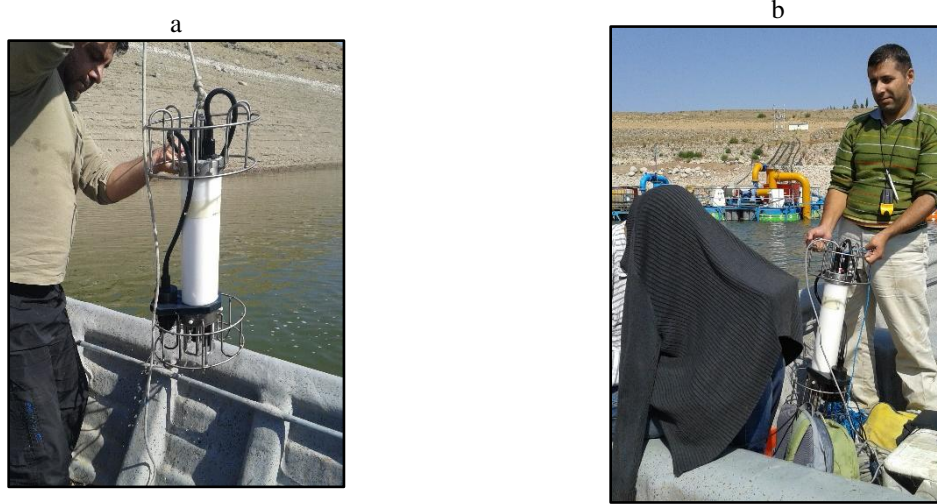
Figure 2. a) Using CTD in Yamchi reservoir; b) Reading CTD data on the boat
