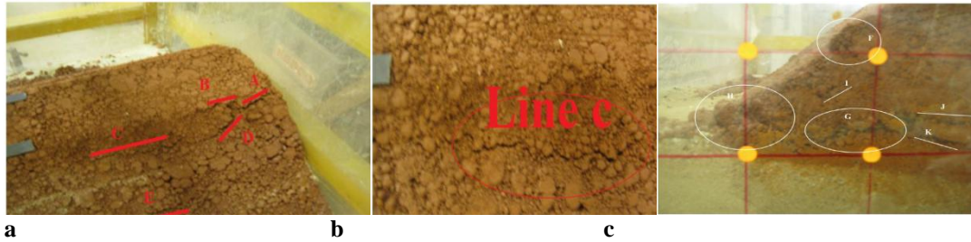
Figure 11. Damage in the first model (Model-A)
