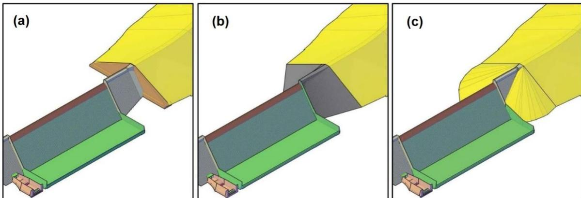
Figure 2. Three methods of transition designing from Rigid part to Embankment Part
