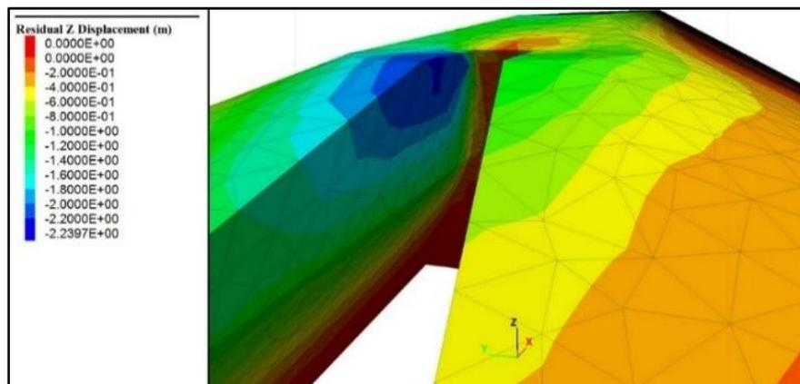
**Figure 9. Residual deformation of the earth-fill dam (MCL, Karebas record)**
