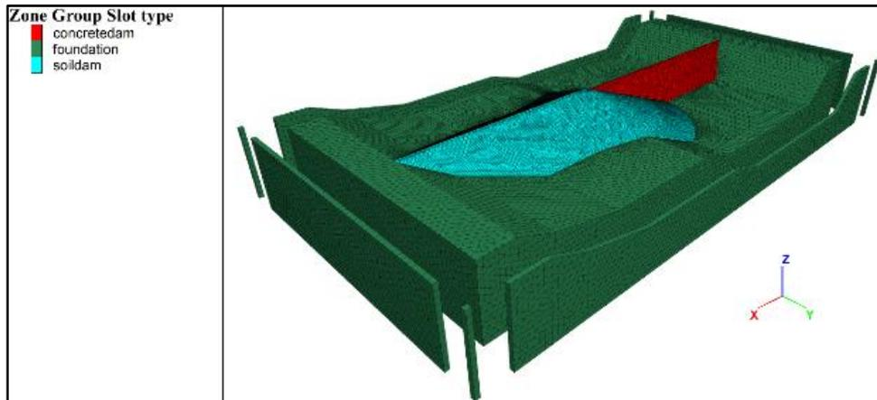
**Figure 7. Absorbent Free-Field boundaries**
