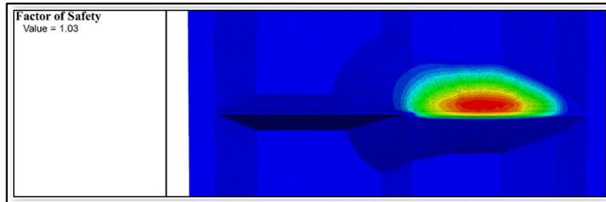
**Figure 8. The minimum safety factor of the critical sliding surface in the Pseudo-Static condition**
