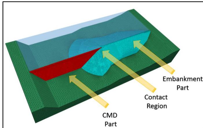
Figure 4. Wrap around method (Dasht-e-Palang Dam)
