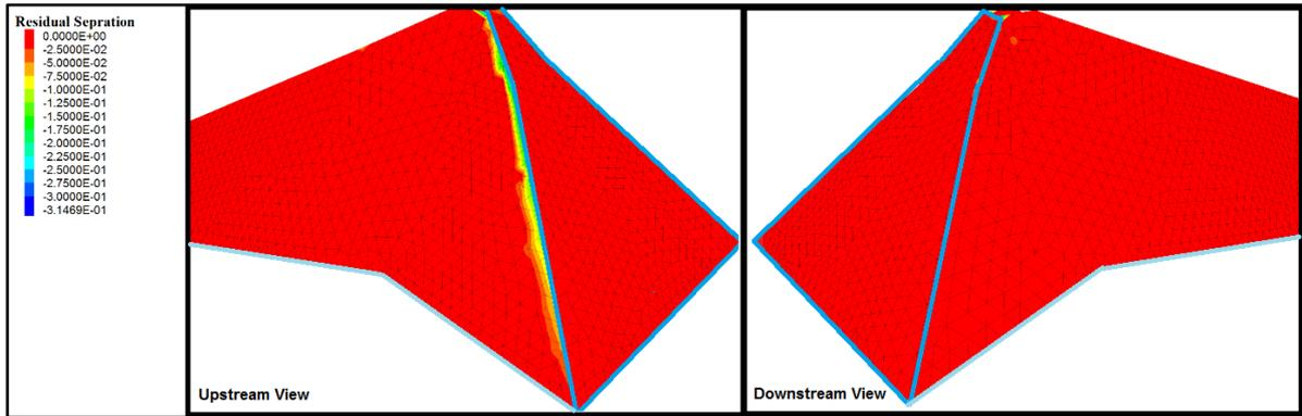
**Figure 10. No Residual separation on clay core bed at MCL**
