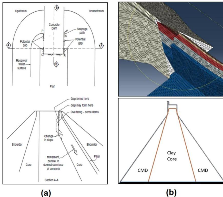
**Figure 6.** (a) Narrow area of RCC for supporting clay core
