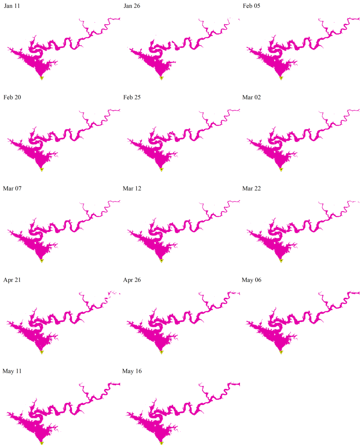
Fig 4. Schematic of water surface area in the Dez Dam between January 11 th and May 16 th , 2019, derived from Sentinel 2 imagery
