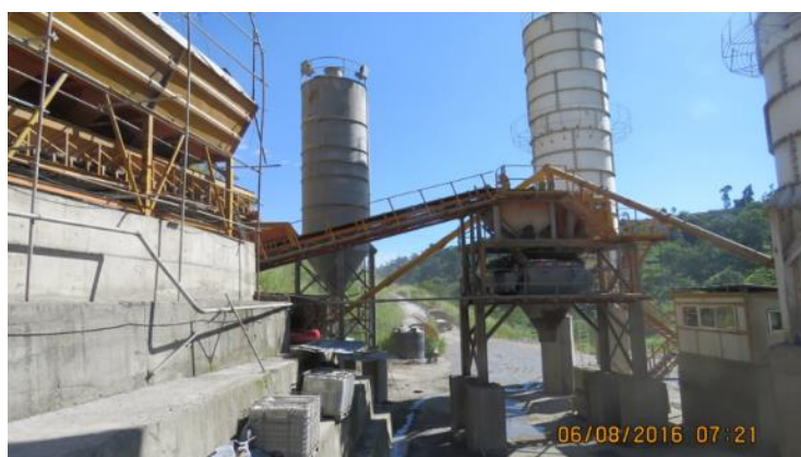
Figure 5. Twin-shaft batching plant mixers with the cement silos
