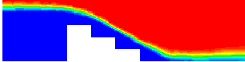
Figure 2. Flow pattern on stepped spillway
