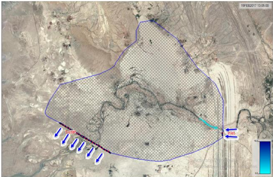
Figure 2 shows the computational grid position and boundary conditions introduced to the two-dimensional model
