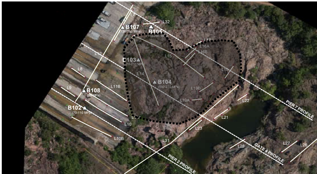
Figure 4 : Plan view of SASW test locations in rock mass downstream of 7-gate spillway.
