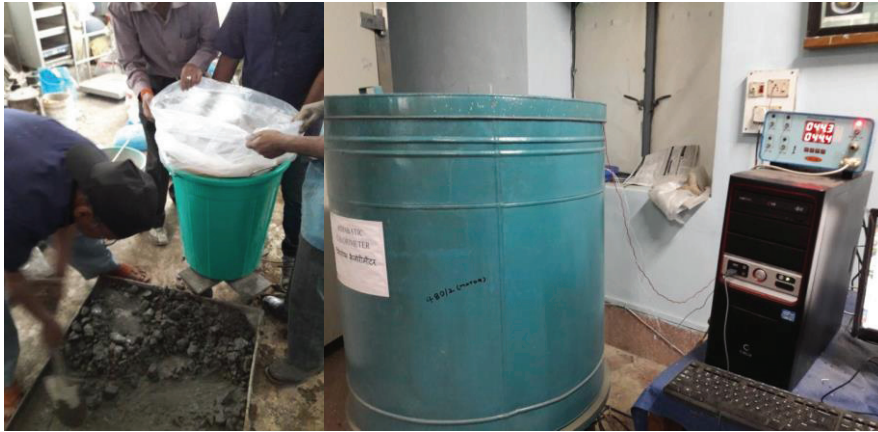
Fig. 4 : Test set up for measuring adiabatic temperature rise
