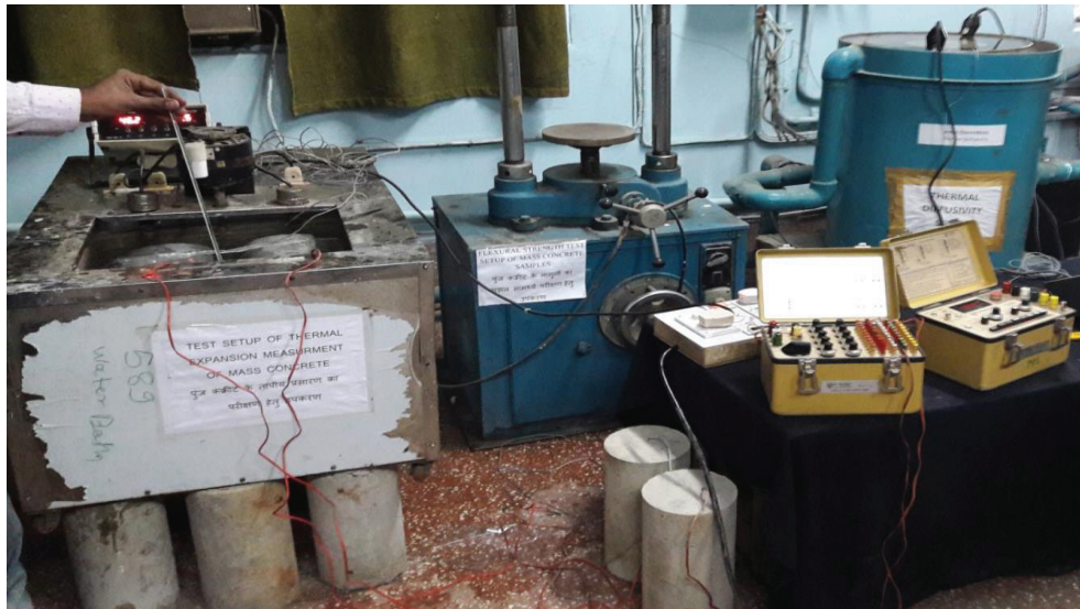
Fig. 8 : Test set up for measurement of Linear Expansion of concrete sample
