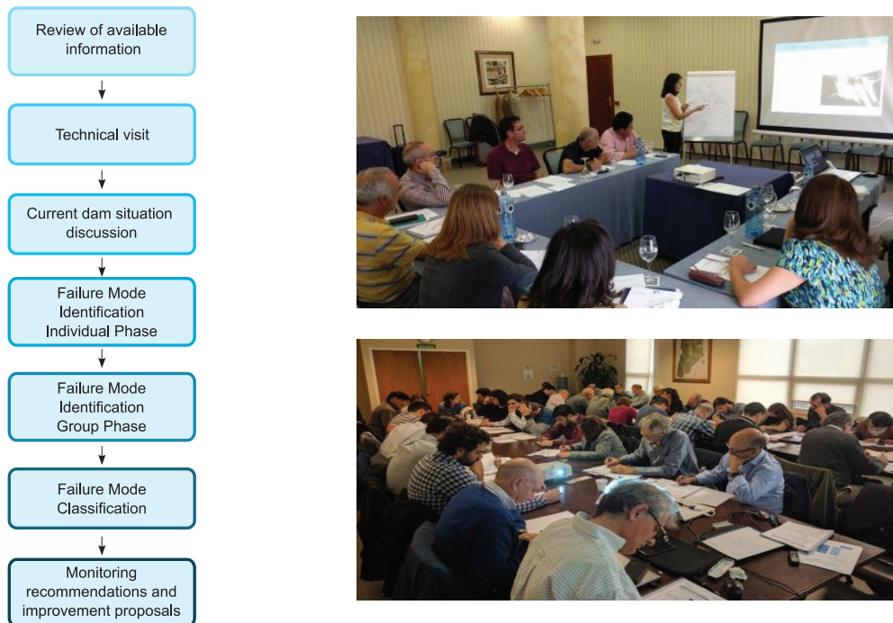
Figure 2 : Steps for technical audit through failure mode identification (left) and pictures of failure mode identification sessions (right).
