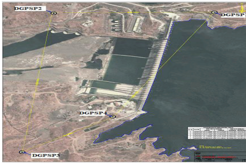
Figure 2 : Control point network at Sardar Sarovar dam
