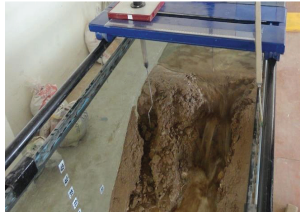
Figure 8 : Headcut erosion of cohesive soil
