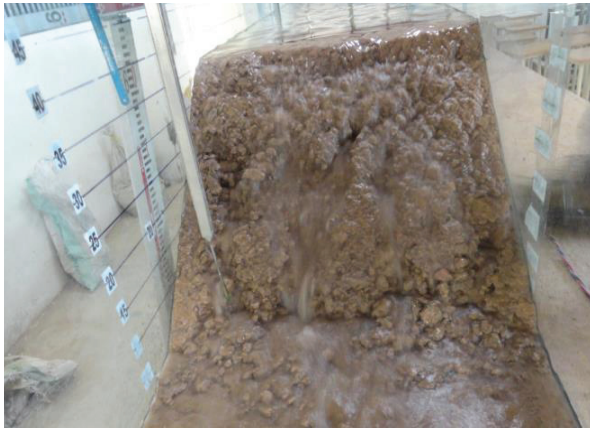
Figure 7 : Surface erosion of non-cohesive soil
