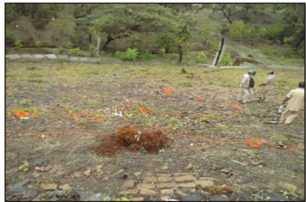
Figure 11 : Locations of Geophones at the downstream face, upstream face of the Vihar dam (Central Portion)
