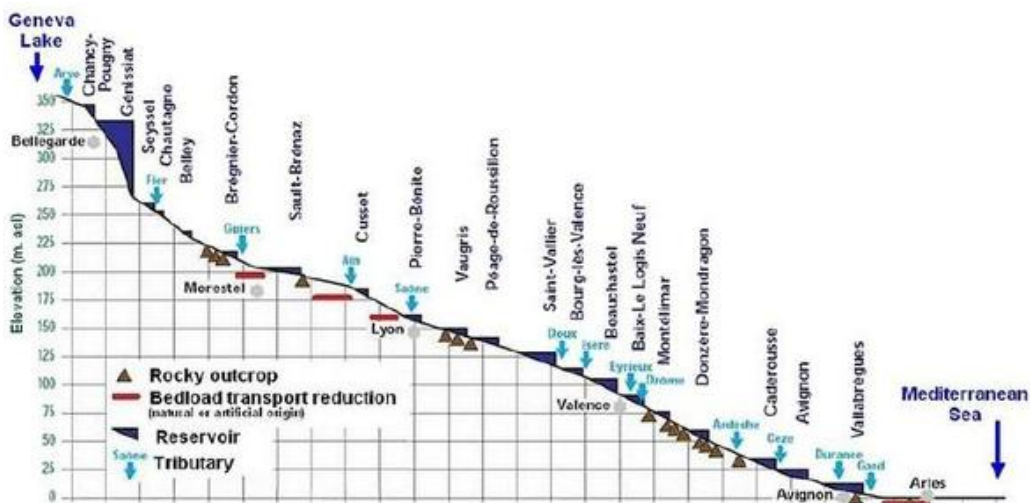
Figure 1. Longitudinal profile of the French Rhone River with cascade of run-of-river power plants (Peteuil 2012)
