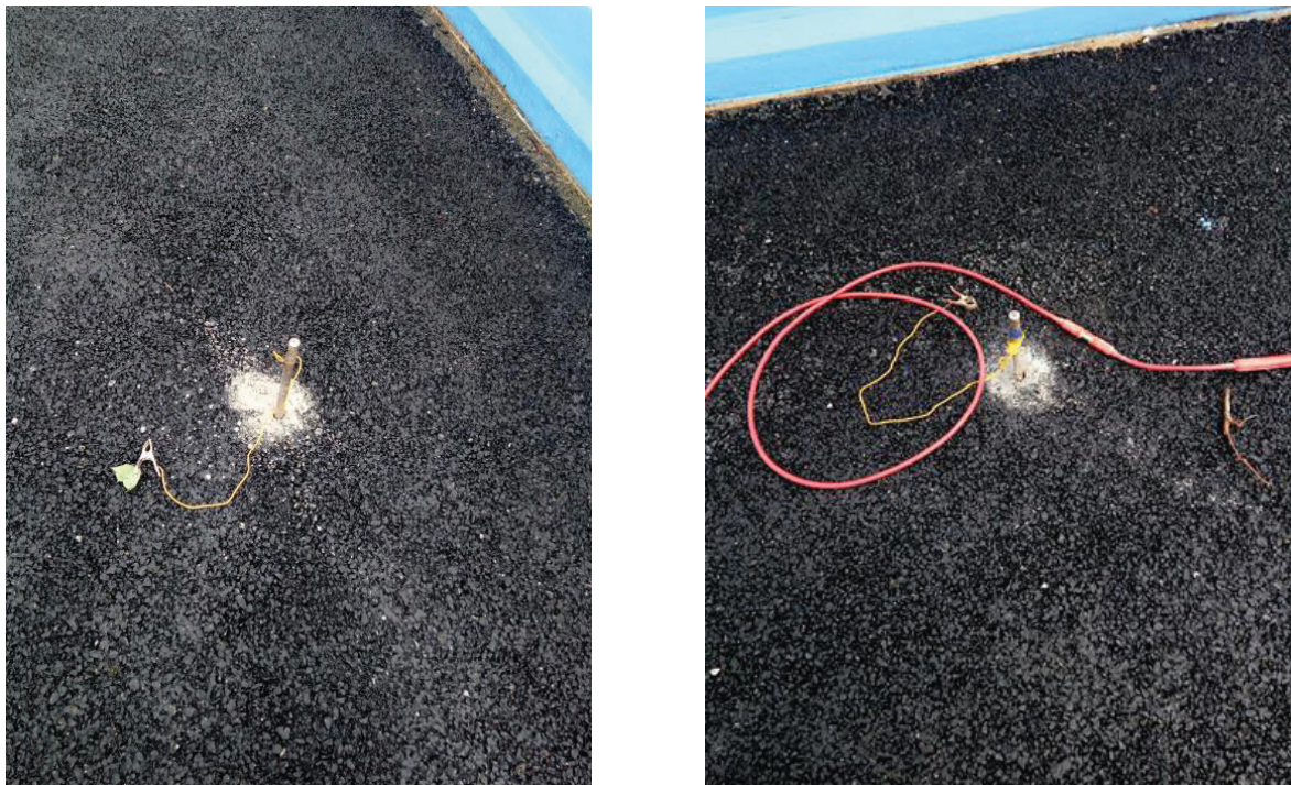
Fig. 1 : Electrodes planted on dam crest
