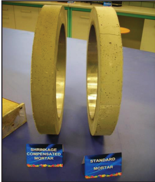
Figure 6 : “O Ring” Test
