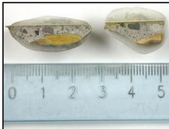
Figure 1 : Colorimetric test with sodium hexanitrocobaltate
