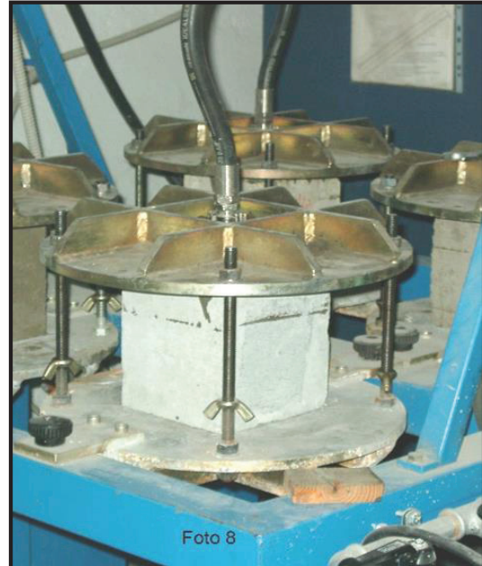
Figure 7 : Water impermeability test
