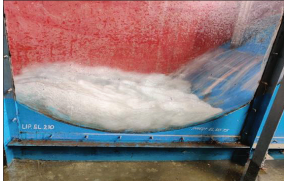
Figure 13 : Gated operation of main spillway with GO 2.5 m (2D model view)
