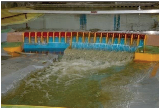
Figure 9 : Ungated operation of main spillway only
