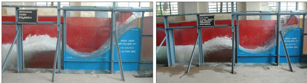
(a) Q = 17,769 \text{ m}^3/\text{s} at FRL El. 262.13 m (b) Q = 35,537 \text{ m}^3/\text{s} at FRL El. 262.13 m
