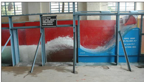
Figure 15 : Gated operation of main spillway with GO 3 m (2D model view)
