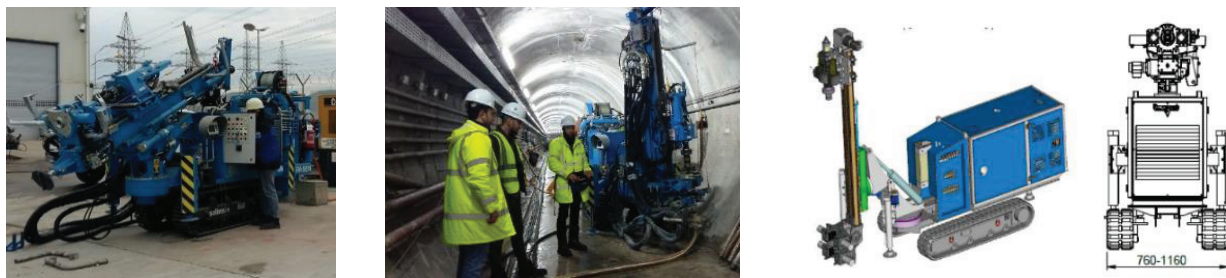
Figure 8 : SoilMec SM-5 EM Drill Rig for Gallery Operation
