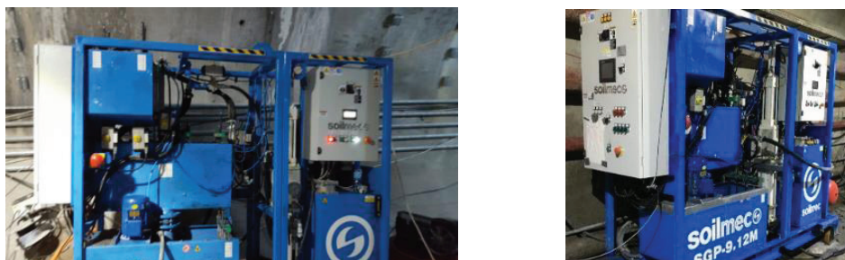
Figure 9 : Soilmec Batching and Grouting Unit (BGU)
