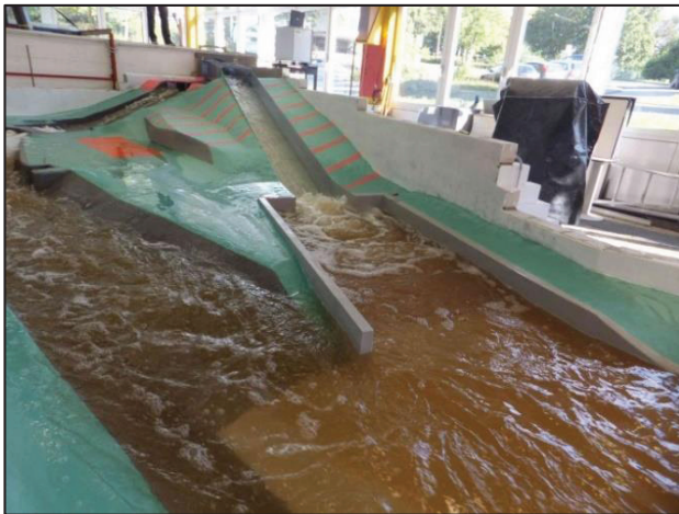
Figure 9 : Hydraulic model scale 1:25
