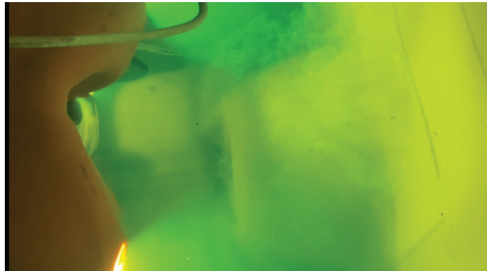
Figure 7 : Dye Injection testing using EyeROV Tuna
