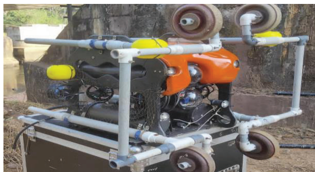
Figure 2 : Customisation for Dam Inspection
