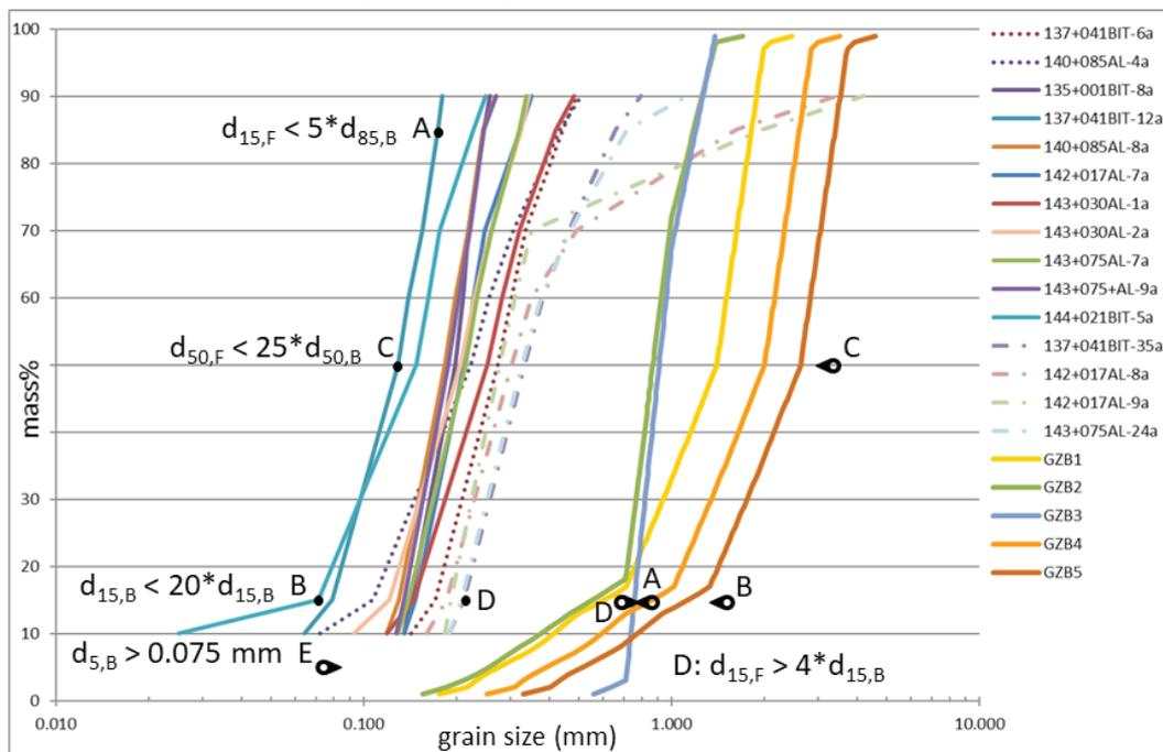
**Figure 3** : Grain size distributions as found in the aquifer at the pilot site and for various coarse sand barrier materials, indicating filter rules applied to the normative distributions (subscript 'F' refers to the filter or barrier material, subscript 'B' to the base or background material).
