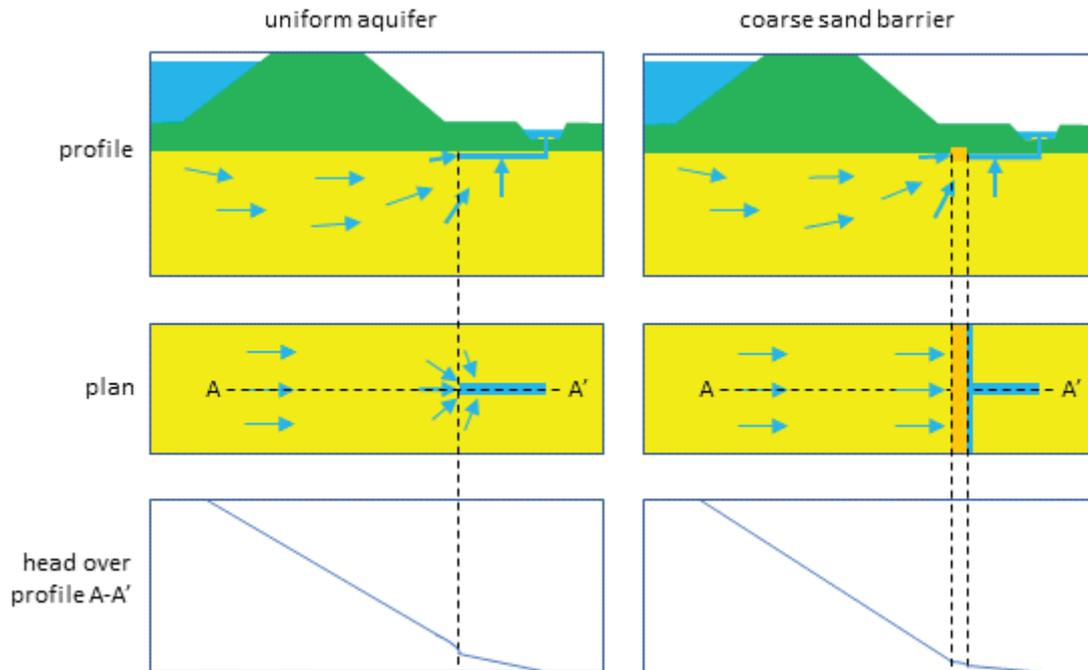
**Figure 1** : Concept of the coarse sand barrier: situations without and with a barrier (Rosenbrand et al., t.b.p.).
