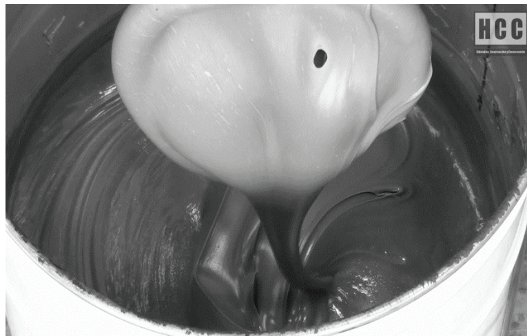
Figure 1 : High viscous-thixotropic putty flowing. Viscosity can be one million times more than water.
