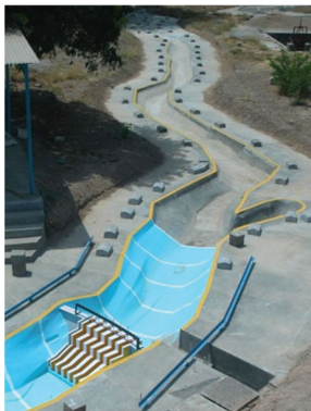
Figure 8 : View of model reach from dam axis to full reach & Figure 9 : Simulation of suspended sediment - View of model near dam and Intake. (Q = 1500 m 3 /s, 3500 ppm, FRL)
