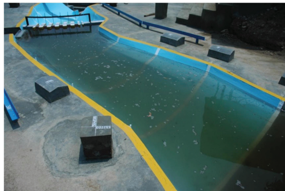
Figure 8 : View of model reach from dam axis to full reach & Figure 9 : Simulation of suspended sediment - View of model near dam and Intake. (Q = 1500 m 3 /s, 3500 ppm, FRL)
