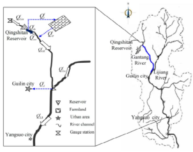
**Fig. 1 :** Schematic of water distribution from the Qingshitan Reservoir (Adapted from Chen et al., 2012).
