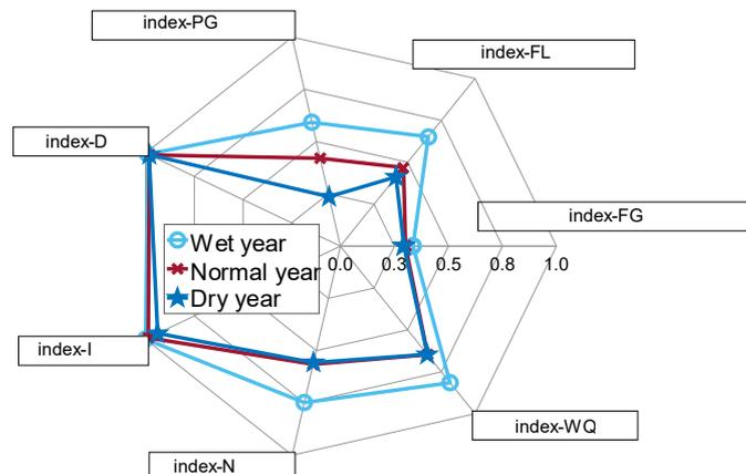
Fig. 4 : Index results of Qinshitan Reservoir under RBM for the three typical years
