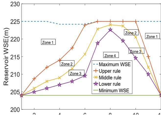
Fig. 2 : Illustration of Rule curve for Qingshitang reservoir operation.
