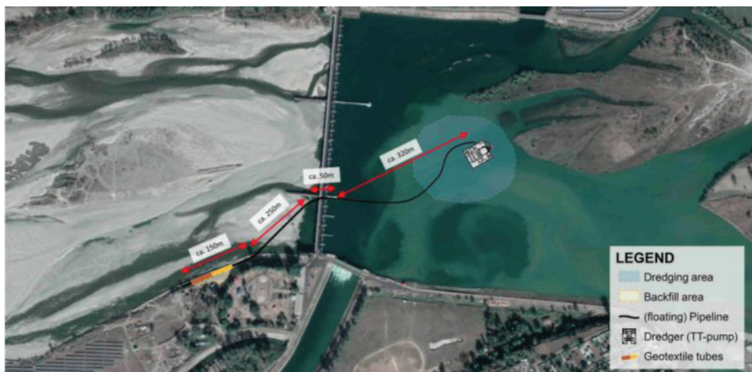
Figure 10 : Dredging, transport and dumping arrangement.
