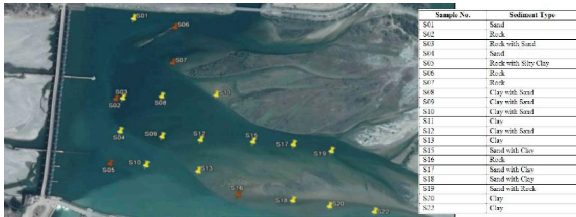
Figure 3 : Location of sediment samples in the Dakpathar Reservoir (the placemarks with dark brown colour indicate rocky areas).
