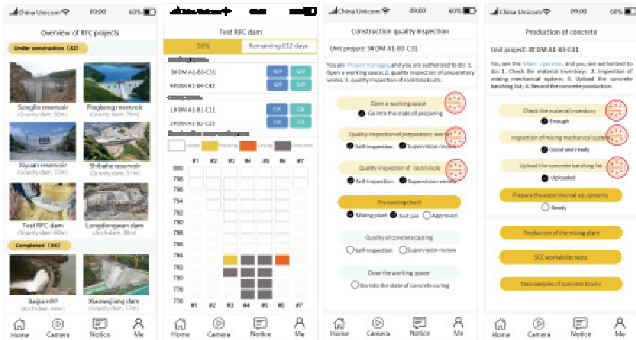
(a) Project list (b) Construction progress (c) Procedure control (d) Concrete production (Note: DM-dam monolith; WP-working space; MP-mixing plant; CR-concrete curing; CB-concrete blocks)
