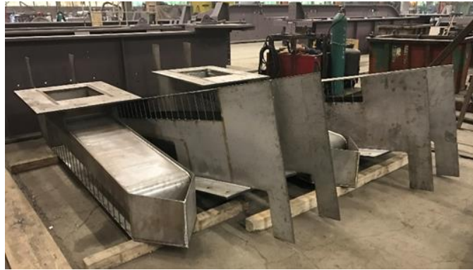
Fig. 13 The production of the steel Fusegate components F..
