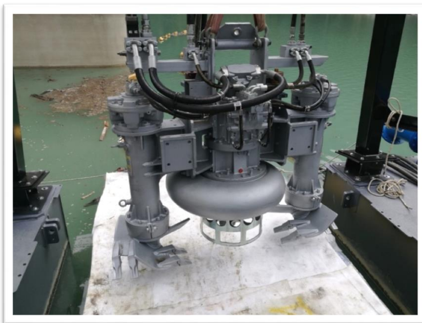
Figure 4. Centrifugal slurry pump with side excavators
