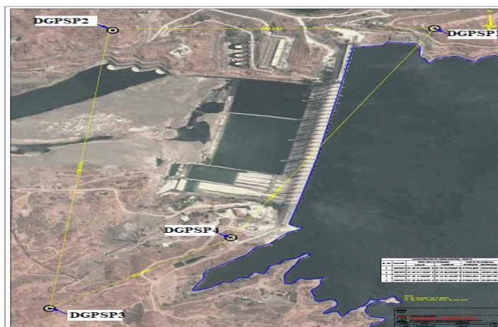
Figure 2. Control point network at Sardar Sarovar dam
