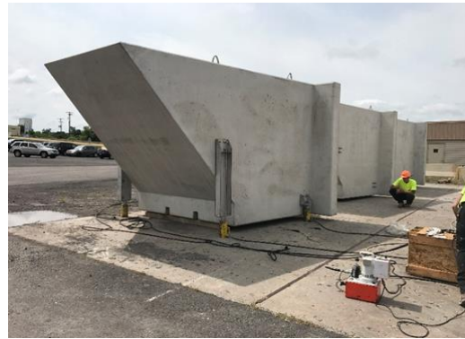
Fig. 12 Fusegate jacking to verify ballast requirements F..
