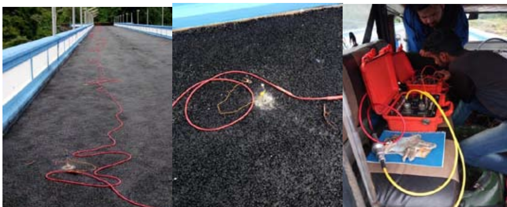
Fig. 4 : Arrangement for ERI on a dam top.
